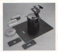
For the analysis of powders or films, a MiniGrip pressure device is included to provide maximum sample contact with the crystal surface. The powder retention ring minimizes the risk of getting powders inside the accessory and sample compartment. This accessory is baseplate mounted for maximum sampling reproducibility.
